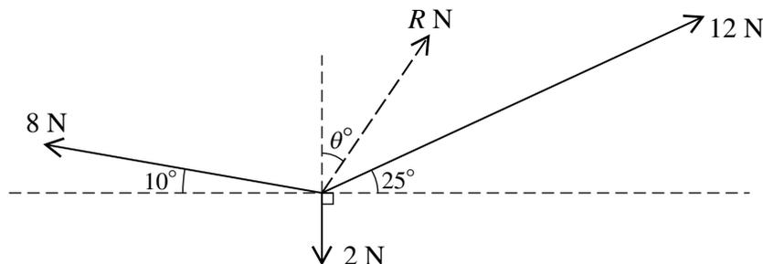
Three coplanar forces of magnitudes  $8 \text{ N}$ ,  $12 \text{ N}$  and  $2 \text{ N}$  act at a point. The resultant of the forces has magnitude  $R \text{ N}$ . The directions of the three forces and the resultant are shown in the diagram. Find  $R$  and  $\theta$ . [7]
