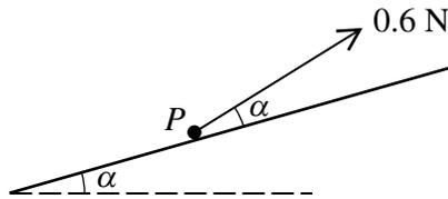
A particle  $P$  of mass  $0.5 \text{ kg}$  rests on a rough plane inclined at angle  $\alpha$  to the horizontal, where  $\sin \alpha = 0.28$ . A force of magnitude  $0.6 \text{ N}$ , acting upwards on  $P$  at angle  $\alpha$  from a line of greatest slope of the plane, is just sufficient to prevent  $P$  sliding down the plane (see diagram). Find
