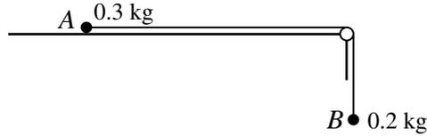
Particles  $A$  and  $B$ , of masses  $0.3 \text{ kg}$  and  $0.2 \text{ kg}$  respectively, are attached to the ends of a light inextensible string.  $A$  is held at rest on a rough horizontal table with the string passing over a small smooth pulley at the edge of the table.  $B$  hangs vertically below the pulley (see diagram). The system is released and  $B$  starts to move downwards with acceleration  $1.6 \text{ m s}^{-2}$ . Find
